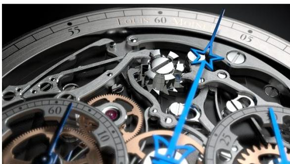
Watchmakers often consider the chronograph to be the finest of watch complications. Comprising a total of over 300 parts, Memoris is perhaps the most spectacular chronograph made to date: its entire function – over 60 parts – is fully visible on the dial side. The three functions of the column wheel, operated by its monopusher, can be seen. The assembly includes two separate hammers, another rare feature. And the swivel of the yoke is
